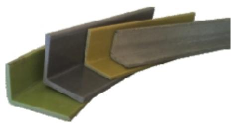
**Armaplast** profiles are manufactured by pultrusion method with combination of plastic resin and continuous glass fiber reinforcement. This continuous process produces composite profiles in rods, tubes and structural shapes. The profiles which are electrical, thermal insulating, uv resistant and fire retardant, are ideally suited for applications where strength and corrosion resistance are required.
